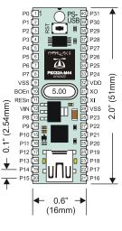
The PropStick USB is suitable for all new Propeller-based designs, whether prototype or production. PropStick USB mounting possibilities include breadboard, perfboard with wire-wrap, or in a 600 mil 40-pin socket soldered to a PCB.
